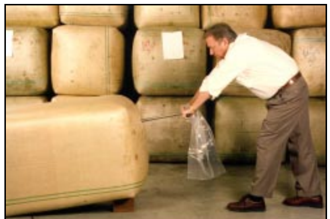
Figure 5: This illustration shows how a bale can be cored without arranging the bale in a block and without standing on the top of the bale. This method is particularly suitable where there is adequate space and the floor surface is sufficiently smooth to allow the bales to be brought to the sampler by hand truck. Note how the sampler positions himself so that the thrust into the bale is made using the arms and shoulders rather than the back.
