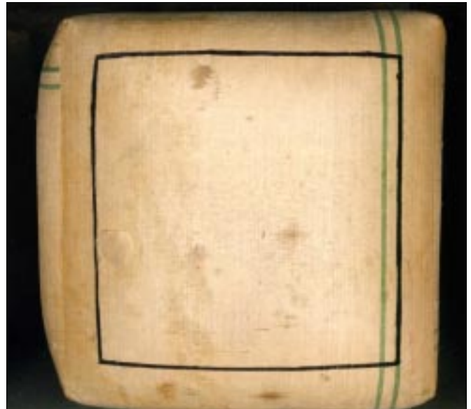
Figure 4: The black line encloses the area within which coring must occur. The edges of the bale represent an area of moisture instability. The core tube should not be allowed to penetrate the bale within 75 mm (3 inches) of its edge.
