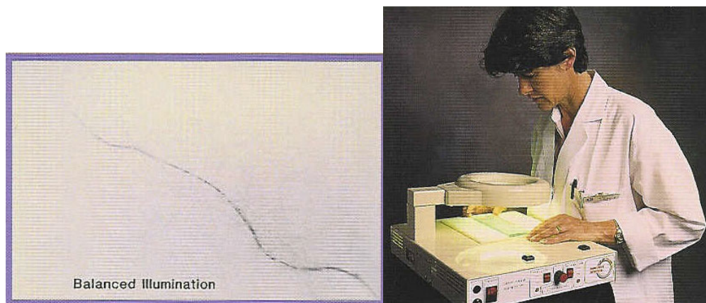
Figure 8 Balanced illumination of the CSIRO Dark Fibre Detector (Source: CSIRO 6 )
