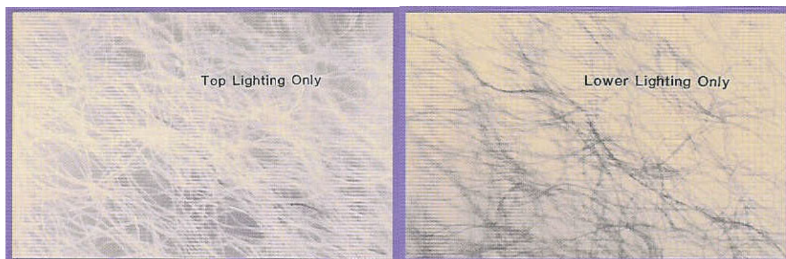
Figure 7 The illumination of a web using top lighting (left) and lower lighting (right) (Source: CSIRO 6 )
