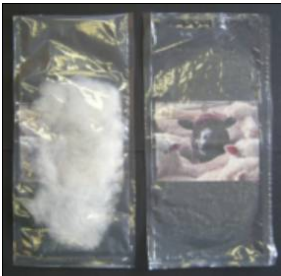
The lower section of the bag contains the wool fibres totally immersed in the solvent in a thin and relatively uniform layer. The wool sliver becomes transparent (right hand image).
