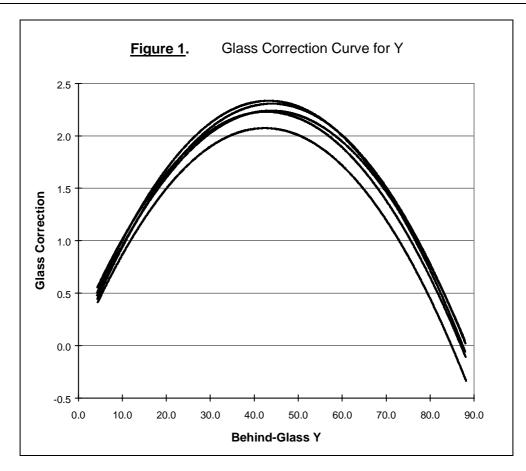
**Table 4:** Glass correction equations (C) that enable 'behind-glass' measurements (x) to be converted predicted 'against-port' values.
